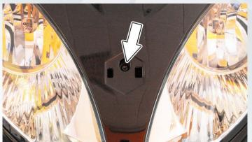
Undo the screws "A" fastening the front grille
