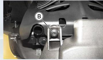
On both sides of the vehicle, undo the screws
