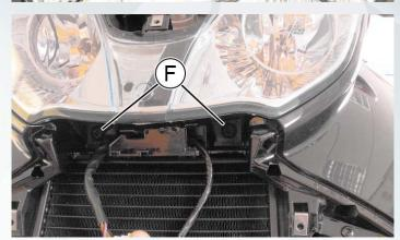
Undo the indicated screws and remove the windscreen
